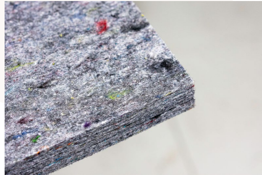
Our sound-absorbing material Re:fill is an example of how we use waste fabric to create new products.
